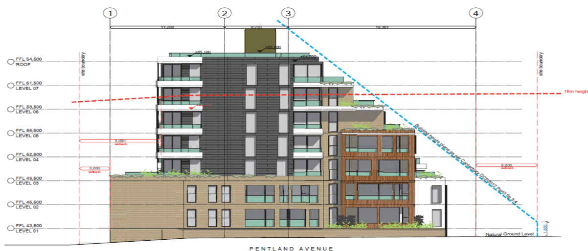
Figure 4: Side view of proposal. Note the stepped design of the rear elevation aimed to reduce overshadowing and privacy impacts to properties to the rear.
